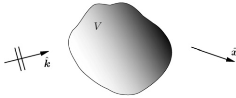
Figure 1. Illustration of the scattering problem. The scatterer V is subject to a plane wave incident in the \hat{k} -direction.
